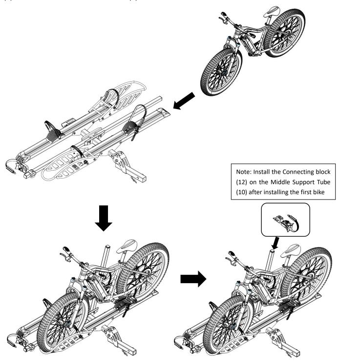
(2). Use the straps from the Front Wheel Holder (6), Crossbeam (5) and Middle Support Tube (10) to fix bike.
