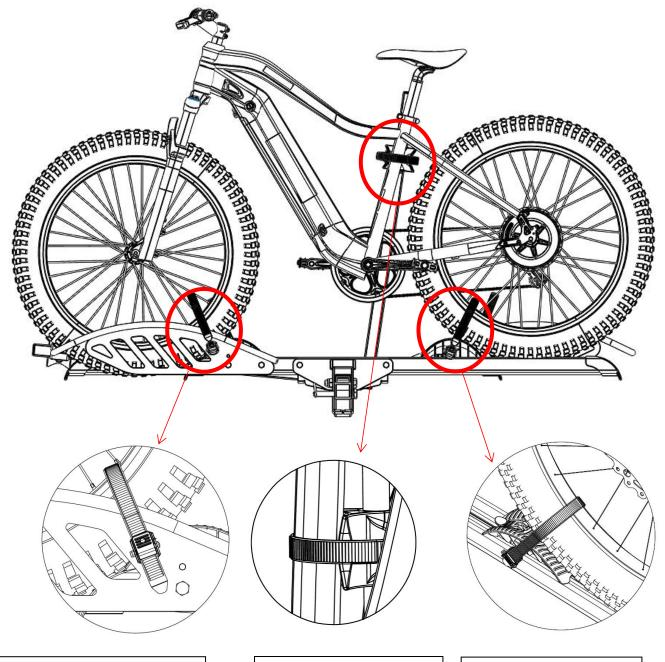
Note: Tighten the straps from the Front Wheel Holder.
