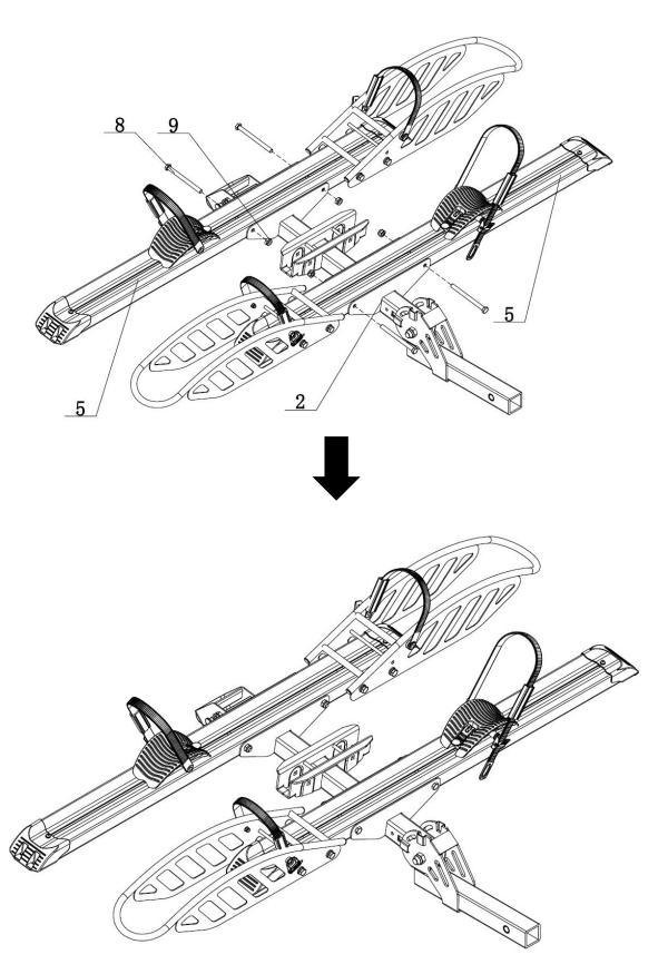
**Step 4**: Insert Middle Support Tube (10) into the base of Bottom Fixing Bracket (2), at the same time, insert the half round gasket (17) from the bottom up to the middle of the square tube and the bottom
