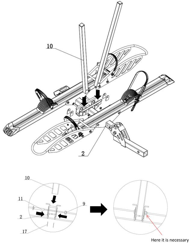
Here it is necessary to reach a torque of 50Nm so that the square tube does not shake.
