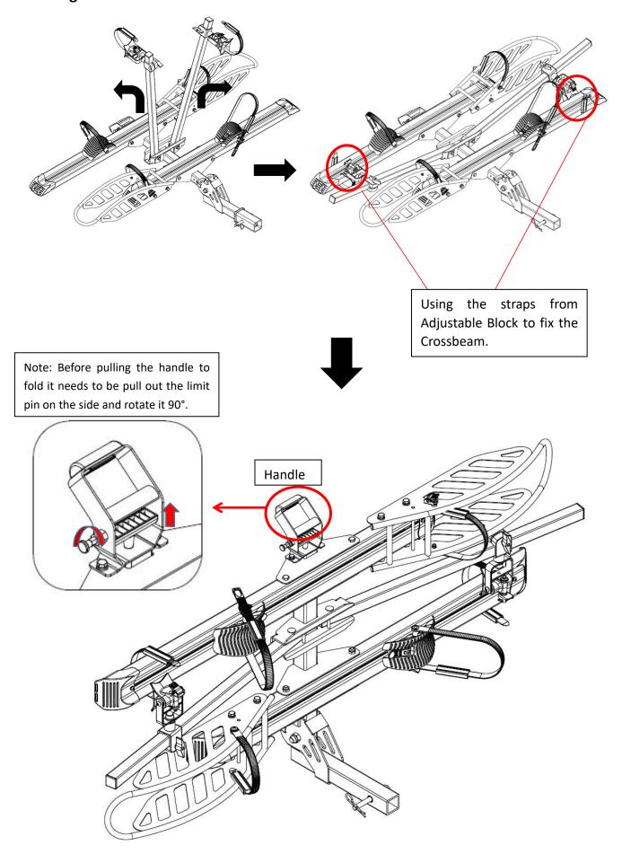
Pull the handle in the direction the arrow shows to fold the bike rack vertically, or to unfold it so it sits flat. The bike rack will automatically stop when it reaches a fixed position
